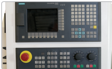
Control Panel: Siemens 808D CNC
