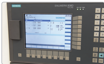
Control Panel: Siemens 808D CNC
