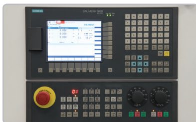
Control Panel: Siemens 808D CNC
