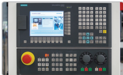
Control Panel: Siemens 808D CNC
