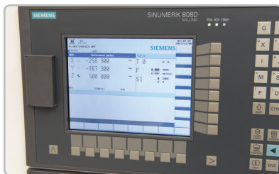
Control Panel: Siemens 808D CNC
